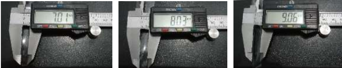
Figure 4. Bottle strips that have been cut at a thickness of 7, 8 and 9 mm.
